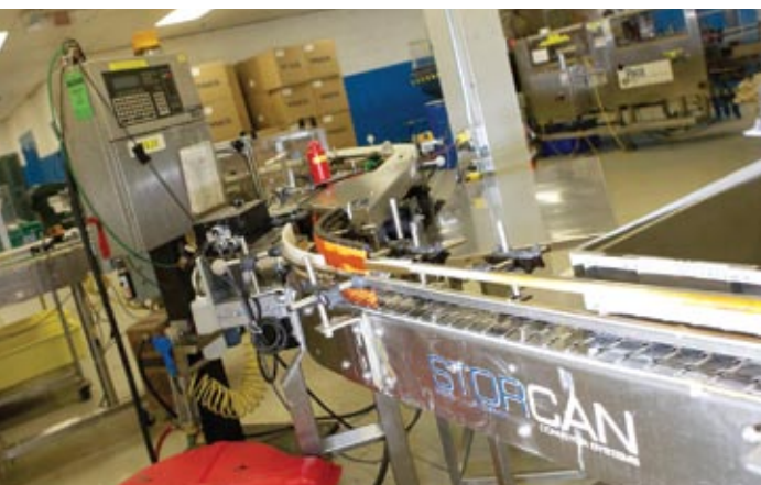
A Storcan conveying system moves personal-care products past a Videojet inkjet coder at the LEK production plant in Knowlton.
