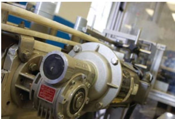
A Bonfiglioli motor helps power a deodorant-stick conveying line.
