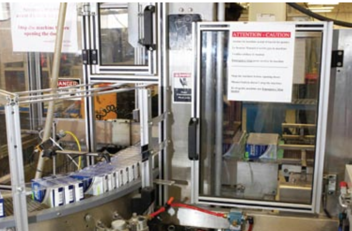
LEK uses a Nenotech SWT30 sleeve wrapper and heat-tunnel to pack cartons of aerosol spray-cans.
