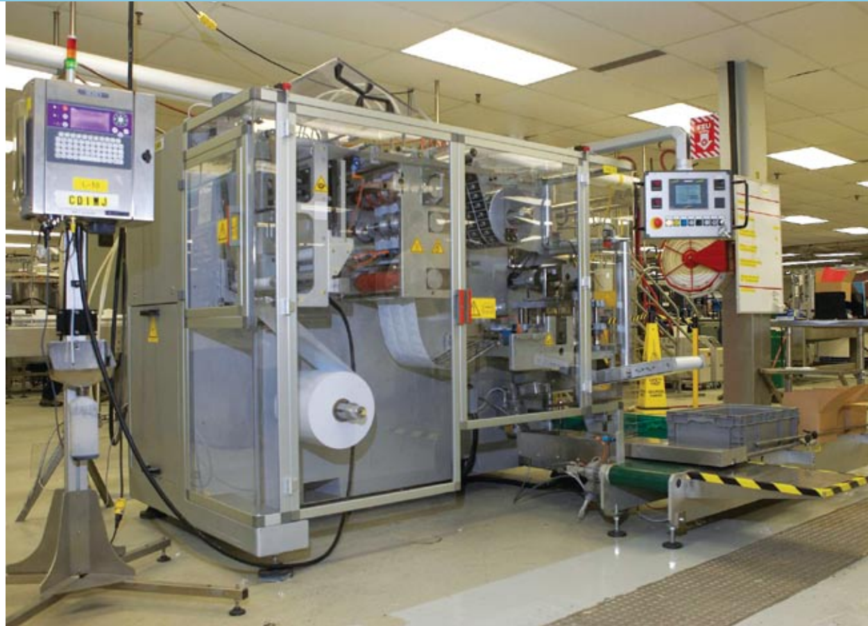
The LEK facility in Knowlton, Que., utilizes a Markem-Imaje 9030 coder to apply lot and best-before information to the web stock of Butterfly sachets being processed on the EasyPack Solutions' Easysnap filling and sealing machine.
