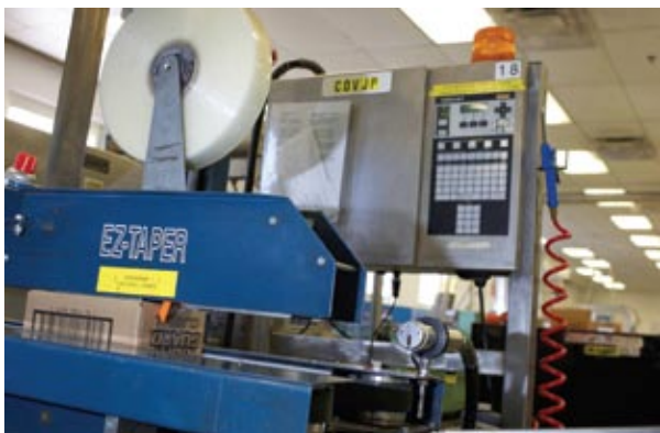
Finished product is cartoned and taped by an EZ-Taper machine, with lot and best-before dates instantly applied by a Videojet model 37e continuous inkjet printer.
