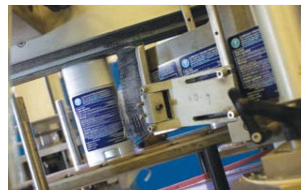
An NJM/CLI 125 Bronco labeler in action on a deodorant line at LEK.
