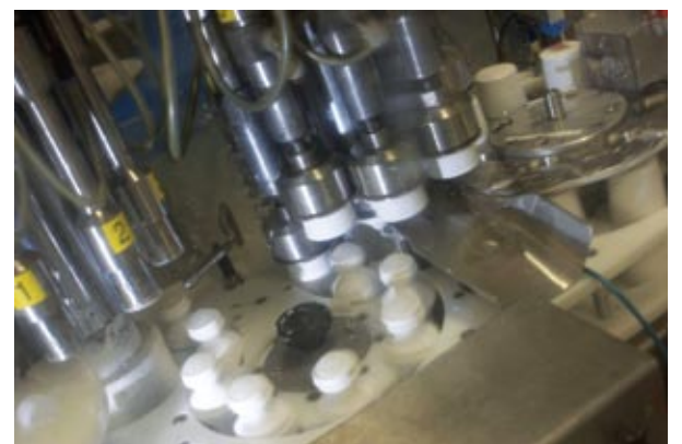
A Capmatic Conquest filler-and-capper employed on the antiperspirant line at the LEK production facility in Knowlton.
