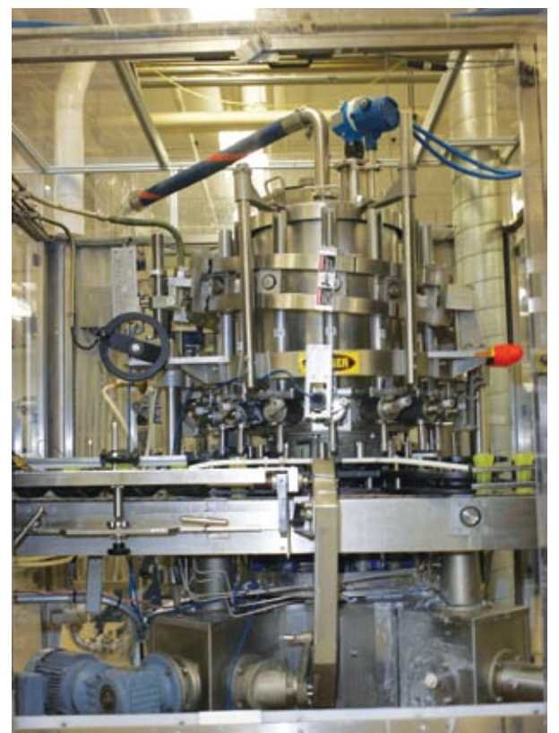
SEW motors help power an Elmar filler on LEK’s liquid soap line.
